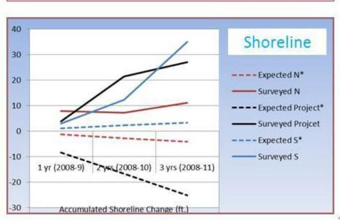
In all of the graphs the South control area (solid blue line) are doing better than historic data (dotted blue line). This indicates no downdrift erosion. Instead downdrift accretion is observed, which is a typical effect of PEM
