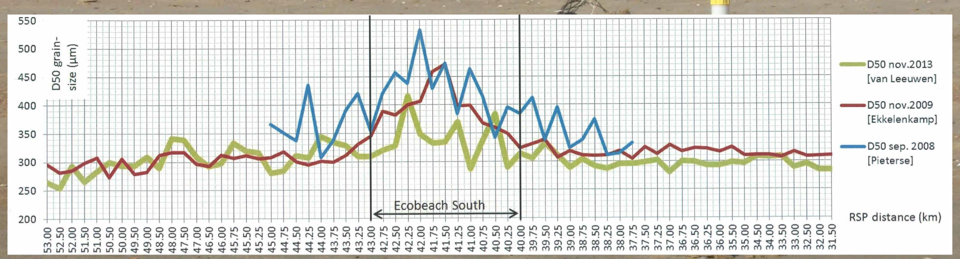
Grain size D50 during and after the Dutch Ecobeach pilot
