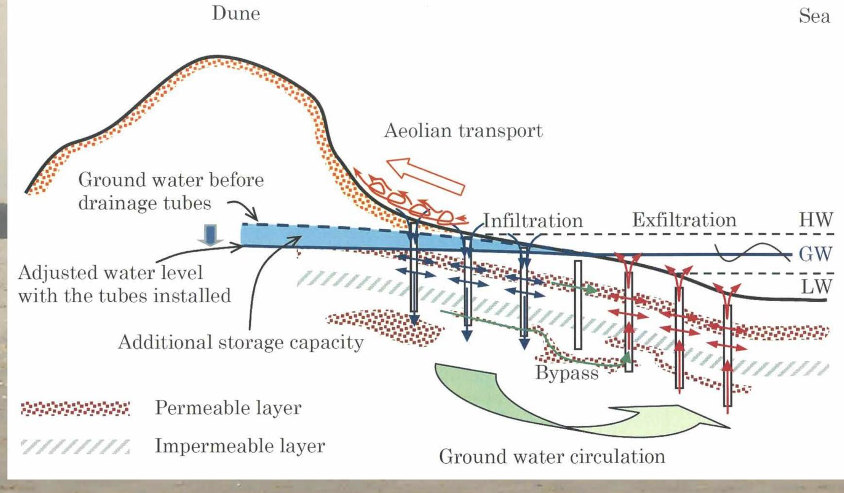
The working mechanism of Ecobeach (Ekkelenkamp 2011)
