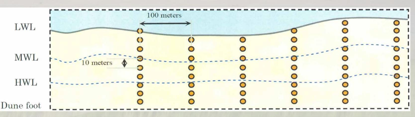
Placement grid of Ecobeach drains
